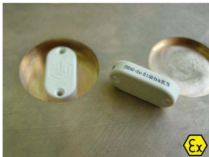
Figure 2. Ferroxtag on screw box ATEX certified re-tuned for metal notch applications.
